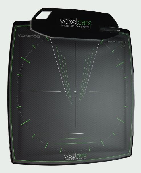
The main component of this foot pressure measuring platform is a quadratic field consisting of 4096 pressure sensors. The data from these sensors is transmitted via a wireless connection to the data modem attached to a computer.
